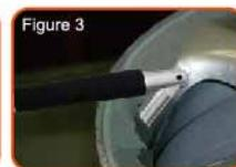
Figures 2 and Figures 3 show a tire service professional properly installing the snap-in valve using the composite tool on an alloy wheel.
