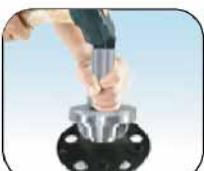
5. Tap the driver handle to face the race or seal into place.
