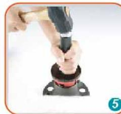
5. Tap the driver handle to force the race or seal into place
