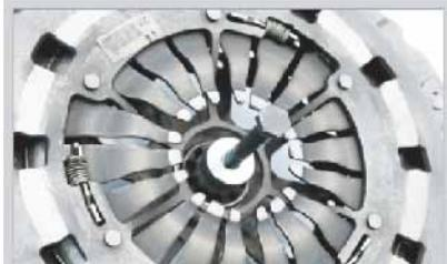
Choose the appropriate centring tool depending on the hub profile diameter of the clutch disc.
