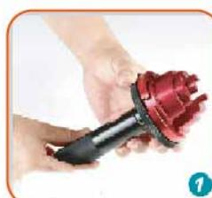
1. Loosen the screw & then turn the dial to expand the jaws.
